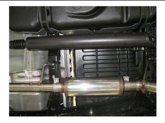
**Step 4.** Next use the supplied 2.50" clamps to attach the Muffler Assembly to the Inlet Pipe and the Tailpipe Assembly to the Muffler Assembly. Complete by fitting the hangers on the Tailpipe into the insulators.
